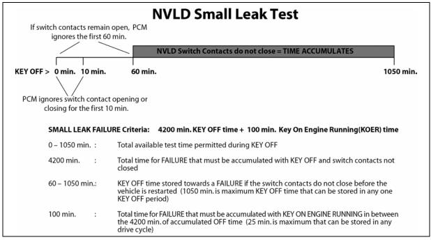
Figure 64 Small Leak Failure Time Thresholds
