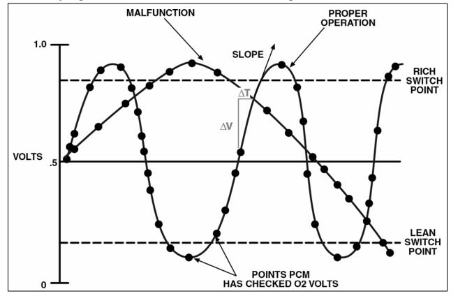
Figure 33 JTEC/SBEC Oxygen Sensor Big Slope
