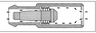
Figure 9 PCV Valve Plunger Front Seated – Low Flow
