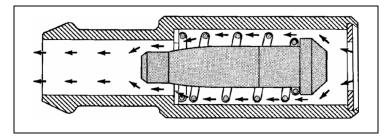
Figure 10 PCV Valve Plunger Mid-Position – High Flow
