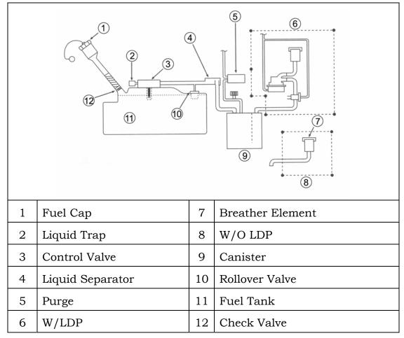
Figure 21 Onboard Refueling Vapor Recovery System
