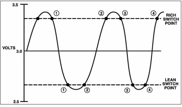
Figure 35 NGC Oxygen Sensor Switch Counts
