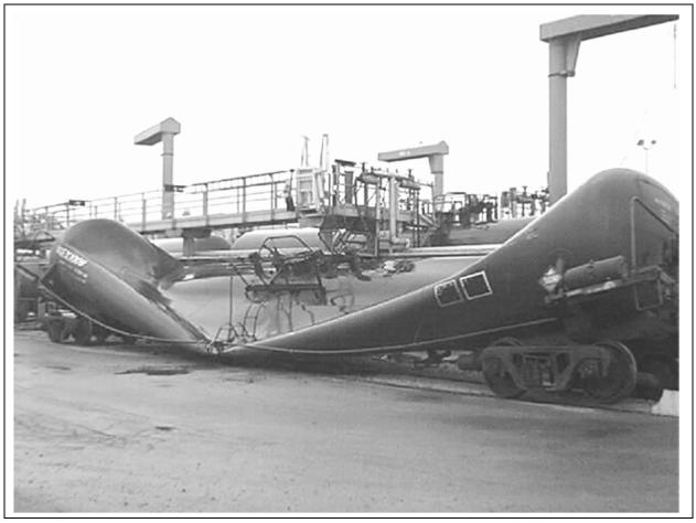
Figure 60 Natural Vacuum Principle Demonstrated
