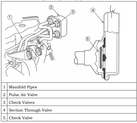
Figure 12 Pulsed AIR System
