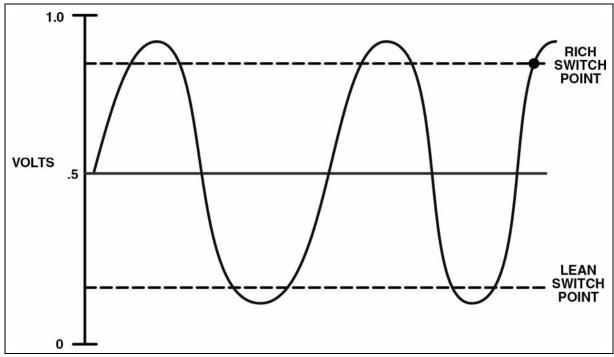
Figure 32 Oxygen Sensor Waveform and Switch Points
