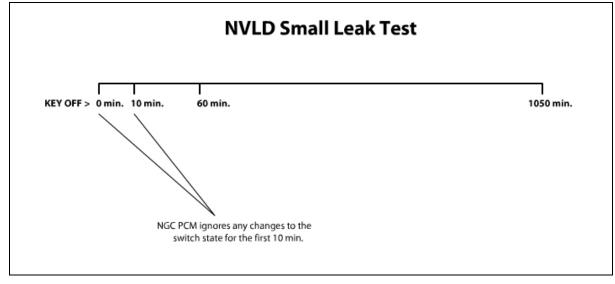
Figure 62 Small Leak Test Main Time Thresholds
