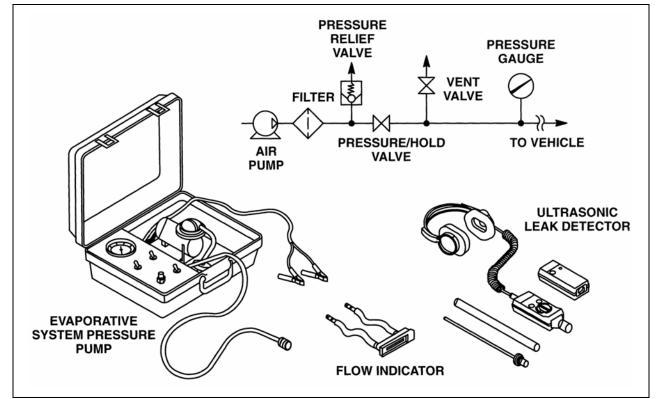
Figure 6 EVAP Pressure Tester and Ultrasonic Leak Detector
