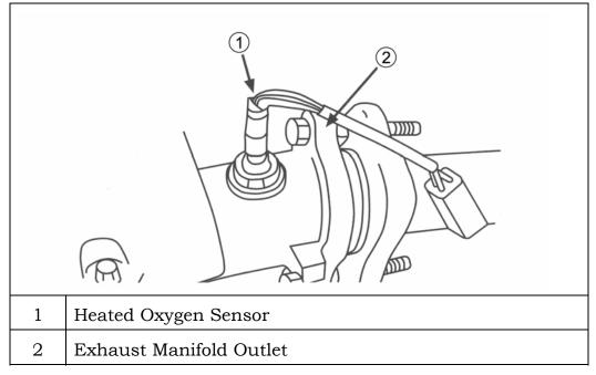
Figure 16 Heated Oxygen Sensor
