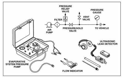
EVAP System Pressure Tester and Ultrasonic Leak Detector
