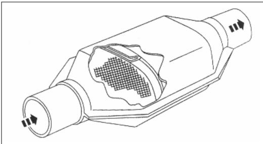
Figure 14 Catalytic Converter
