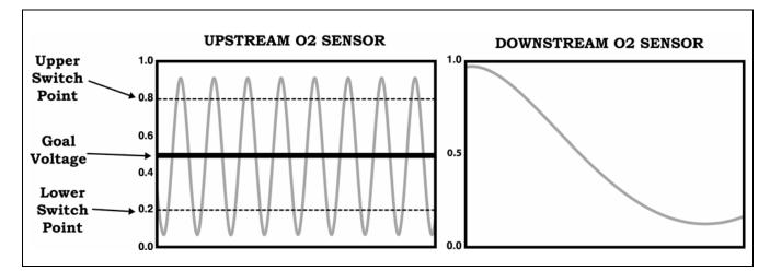
Figure 19 Upstream and Downstream O2 Sensor Signals
