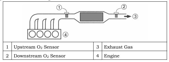
Figure 18 Downstream Oxygen Sensor Location
