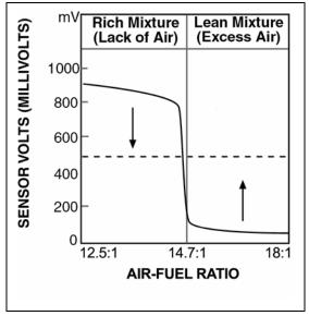
Figure 31 O<sub>2</sub> Sensor Signal
