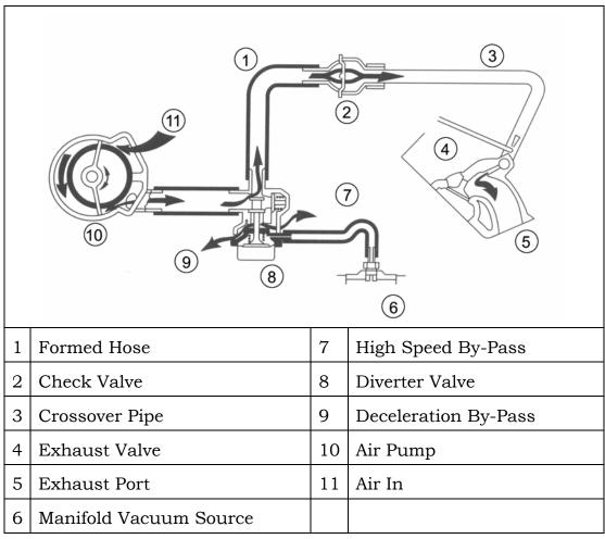
Figure 11 AIR System – Engine Driven Pump
