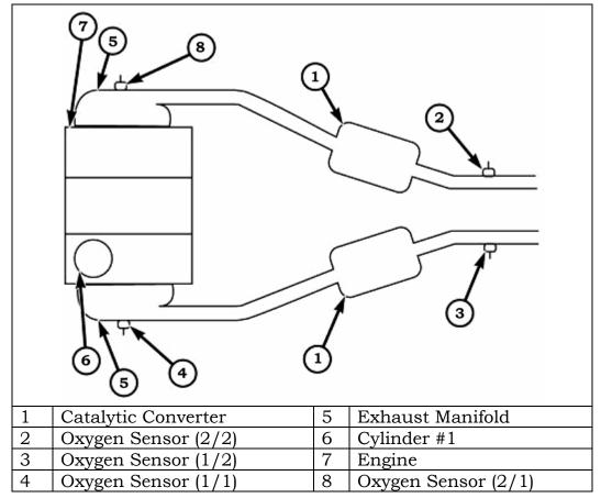
Figure 20 Oxygen Sensor Naming Conventions
