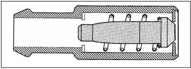
Figure 8 PCV Valve Plunger Back Seated - Closed
