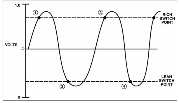
Figure 34 JTEC/SBEC Oxygen Sensor Half Cycles
